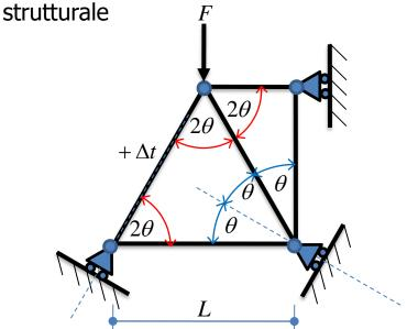
F=1kN; L=1m;  $\theta=30^{\circ}$ ;  $\Delta t=10^{\circ}C$
