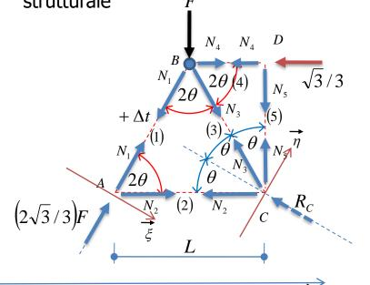
F=1kN; L=1m;  $\theta=30^{\circ}$ ;  $\Delta t=10^{\circ}C$
