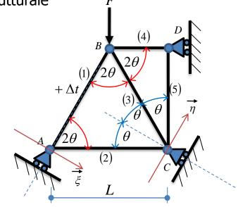
$$\underline{F} = \begin{vmatrix} F_{\xi}^{A} \\ F_{x}^{B} \\ F_{y}^{B} \\ F_{\eta}^{C} \\ F_{y}^{D} \end{vmatrix} = \begin{bmatrix} 0 \\ 0 \\ -F \\ 0 \\ 0 \end{bmatrix} = \begin{bmatrix} 0 \\ 0 \\ -1 \\ 0 \\ 0 \end{bmatrix} kN$$
