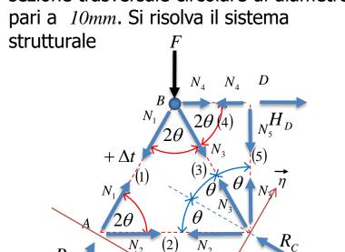
F=1kN; L=1m;  $\theta=30^{\circ}$ ;  $\Delta t=10^{\circ}C$
