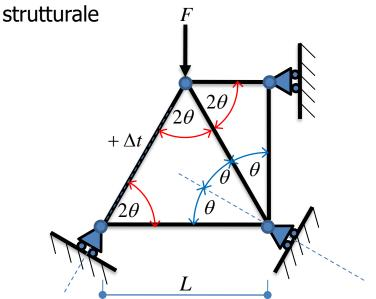
F=1kN; L=1m;  $\theta=30^{\circ}$ ;  $\Delta t=10^{\circ}C$
