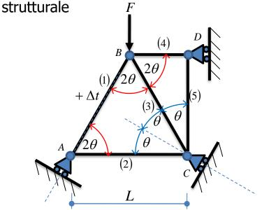
F=1kN; L=1m;  $\theta=30^{\circ}$ ;  $\Delta t=10^{\circ}C$
