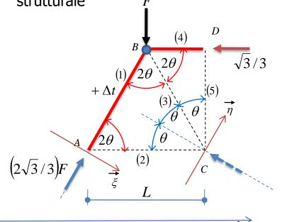
F=1kN; L=1m;  $\theta=30^{\circ}$ ;  $\Delta t=10^{\circ}C$
