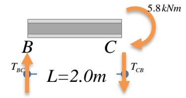
$$\begin{cases} \sum M_{(B)} = 0 \rightarrow T_{CB} L + 5.8 \text{ kNm} = 0 \\ \sum M_{(C)} = 0 \rightarrow T_{BC} L + 5.8 \text{ kNm} = 0 \end{cases} \Rightarrow \begin{cases} T_{CB} = -2.9 \text{ kN} \\ T_{BC} = -2.9 \text{ kN} \end{cases}$$
