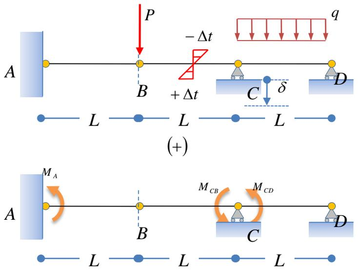
$$\begin{cases} M_{CB} + M_{CD} = 0 \\ M_{CB} \frac{L}{3EI_x} + \frac{v_B - \delta}{L} + \frac{\alpha \Delta t}{h} L = M_{CD} \frac{L}{3EI_x} + \frac{\delta}{L} - \frac{qL^3}{24EI_x} \\ M_A \frac{L}{3EI_x} - \frac{v_B}{L} = 0 \end{cases}$$
