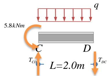
$$\begin{cases} \sum M_{(C)} = 0 \rightarrow 5.8 kNm - T_{DC} L - q L^2 / 2 = 0 \\ \sum M_{(D)} = 0 \rightarrow 5.8 kNm + q L^2 / 2 - T_{CD} L = 0 \end{cases} \Rightarrow \begin{cases} T_{DC} = -7.1 kN \\ T_{CD} = 12.9 kN \end{cases}$$
