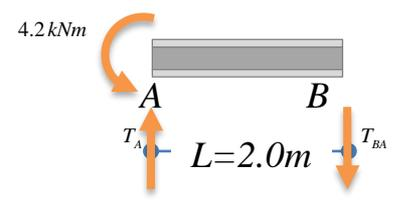
$$\begin{cases} \sum M_{(A)} = 0 \rightarrow -T_{BA} L + 4.2 = 0 \\ \sum M_{(B)} = 0 \rightarrow -T_A L + 4.2 = 0 \end{cases} \Rightarrow \begin{cases} T_A = 2.1 \text{ kN} \\ T_{BA} = 2.1 \text{ kN} \end{cases}$$
