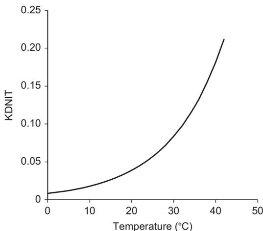
**Fig. 18.6.** Sensitivity (KDNIT) of N denitrification to temperature.
