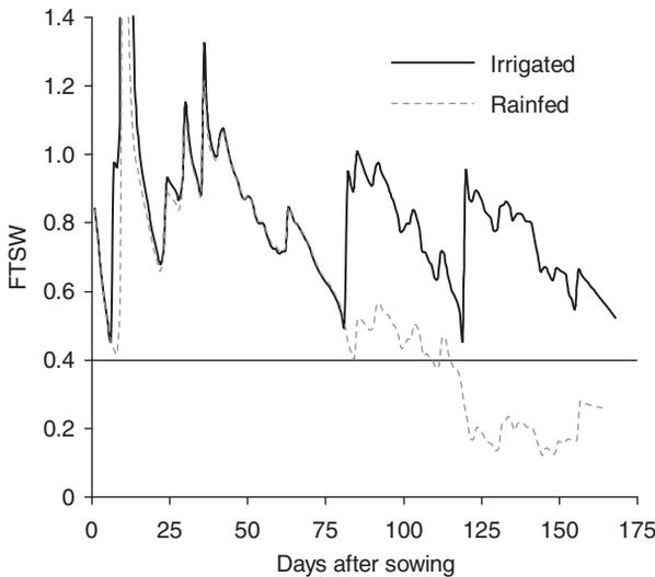
**Fig. 16.3.** Simulated changes in fraction transpirable soil water (FTSW) for wheat in Gorgan during growing season of 2005/06 under irrigated and rainfed conditions. Horizontal line marks FTSW of 0.4, below which crop growth is negatively affected.
