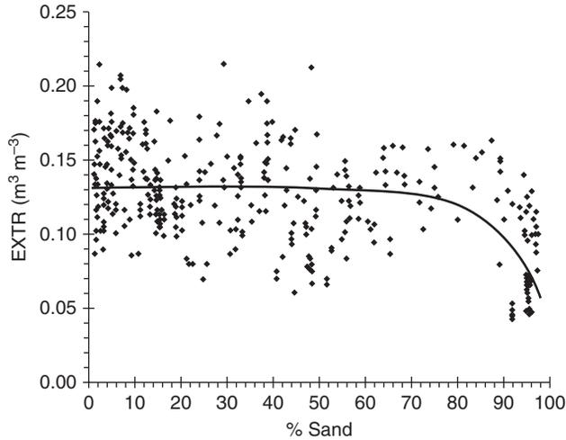
**Fig. 13.2.** Volumetric extractable soil water content as a function of sand percentage ( $x$ ) in the soil. The equation of the line is  $y = 0.132 - 2.5 \times 10^{-6} e^{0.105x}$  (Ritchie *et al.*, 1999).
