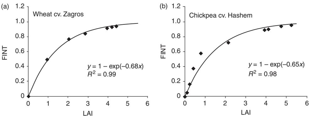
**Fig. 10.8.** Sample fit of Eqn 10.2 to fraction intercepted PAR versus LAI in wheat (a) and chickpea (b). PAR interception has been measured under an umbrella (V. Madah and A. Soltani, unpublished data).
