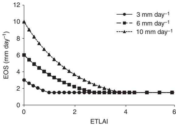
**Fig. 14.6.** Potential evaporation (EOS, mm day<sup>-1</sup>) from soil surface as a function of LAI for calculation of evapotranspiration (ETLAI) for three values of daily potential evaporation of 3, 6, and 10 mm day<sup>-1</sup>.
