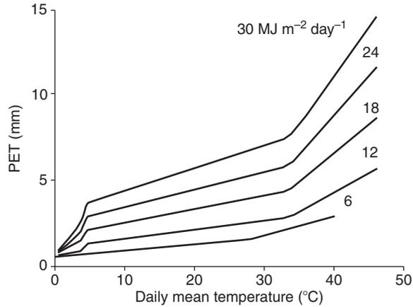
**Fig. 14.9.** Potential evapotranspiration (PET, mm) as a function of mean daily temperature and daily solar radiation ( $\text{MJ m}^{-2} \text{day}^{-1}$ ) calculated using the Priestley and Taylor method.
