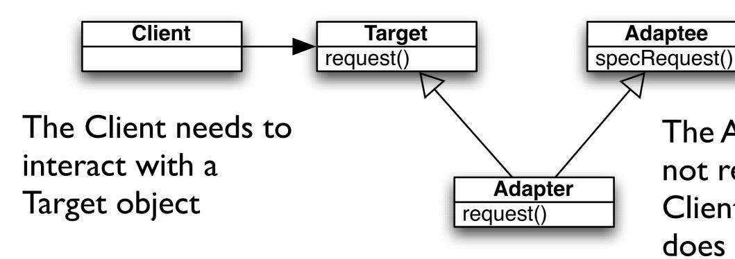
The Adaptee could not respond to Client because it does not have the required method
