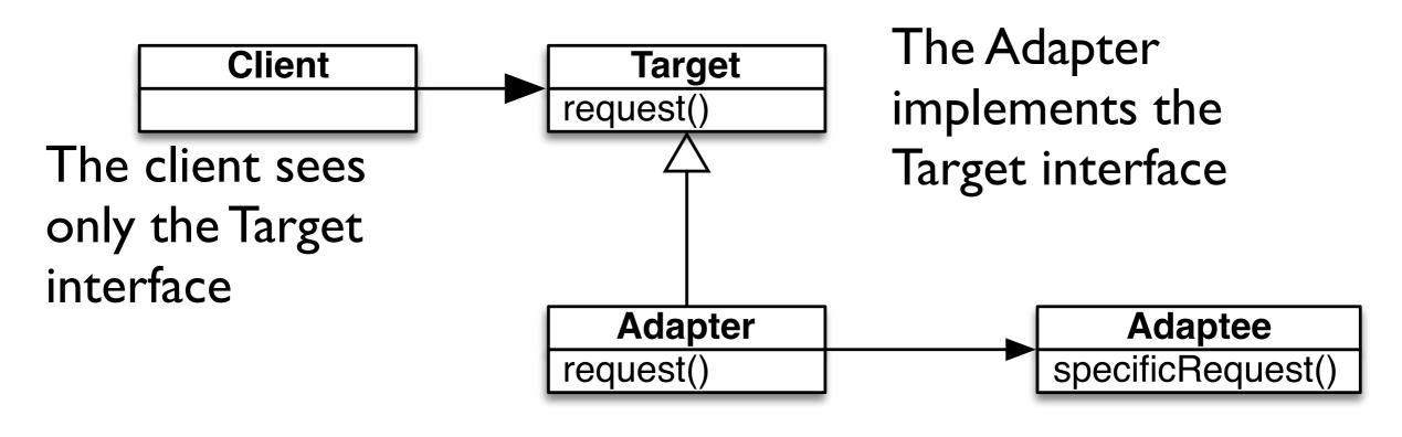
The Adapter is composed with the Adaptee
