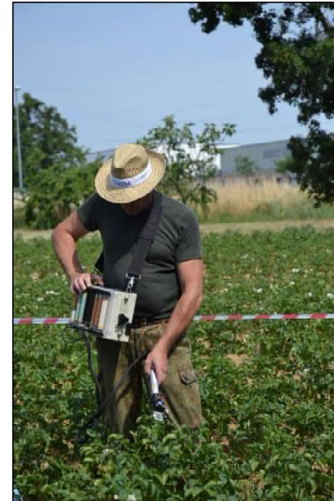
*Portable Photosynthesis System (PPS)
