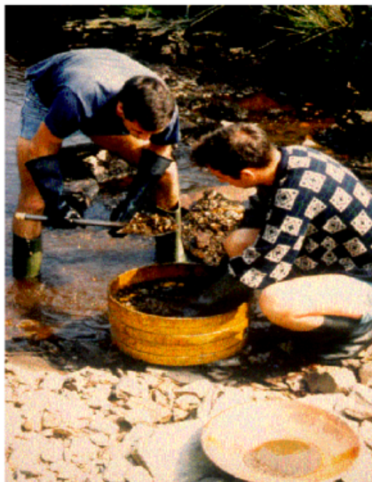
Figure 13. Figure 13. Wet sieving of a stream sediment sample in the UK (Photo: Fiona Fordyce, BGS from Salminen and Tarvainen et al. 1998, Fig. 7, p.21).
