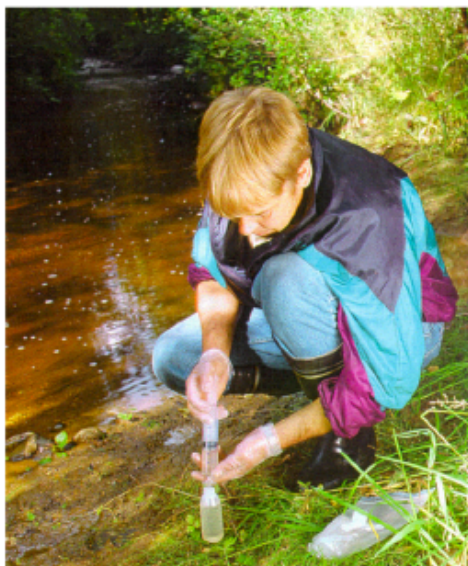
Figure 12. Figure 12. Filtration of a stream water sample (photo: Jari Viitinen, GTK, from Salminen, Tarvainen et al., 1998, Fig. 6, p.17)
