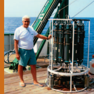
The first author beside the CTD (conductivity, temperature, depth) system used to collect seawater samples at different depths. CO 2 is measured to determine the saturation state of seawater.
