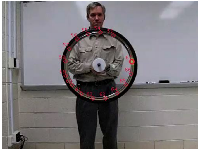
Figure 5.7: Marks for the green sticker on the rotating bicycle wheel.
