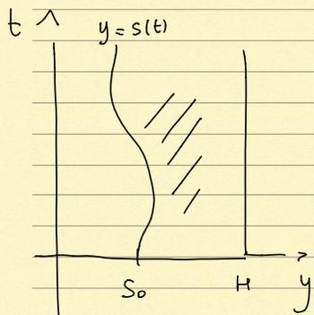
$$\left\{ \begin{array}{ll} \rho v_t = \mu v_{yy} + G & y \in [s(t), H] \quad t \geq 0 \\ v(y, 0) = v_0(y) & y \in [s_0, H] \\ s(0) = s_0 & s_0 \in (0, H) \\ v(H, t) = 0 & t \geq 0 \\ v_y(s, t) = 0 & t \geq 0 \\ v_t(s, t) = \frac{1}{\rho} \left( G - \frac{2b}{S} \right) & t \geq 0 \end{array} \right.$$
