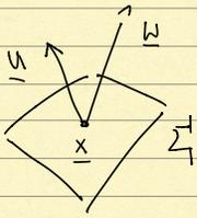
$$\text{flusso att. } \Sigma_1 = \int_{\Sigma_1} \underline{w} \cdot \underline{u} \, d\sigma$$
