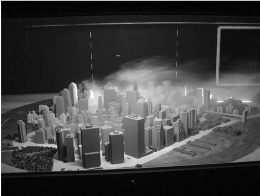
Fig. 22.2. Example of neutrally buoyant smoke released from the WTC physical model, showing flow from left to right is displayed; natural light is illuminating the smoke and a vertical laser sheet is additionally illuminating the plume near the centerline of source. Source: US Environmental Protection Agency. Perry, S., and Heath, D., Fluid Modeling Facility . Research Triangle Park, NC, 2006.
