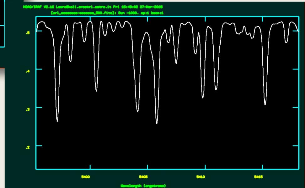
UVES spectrum of the Sun at its original resolution  $R=47000$  and binned to mimic a lower resolution spectrum
