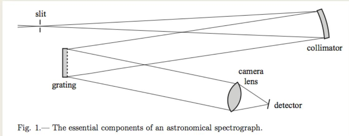
Fig. 1.— The essential components of an astronomical spectrograph.
