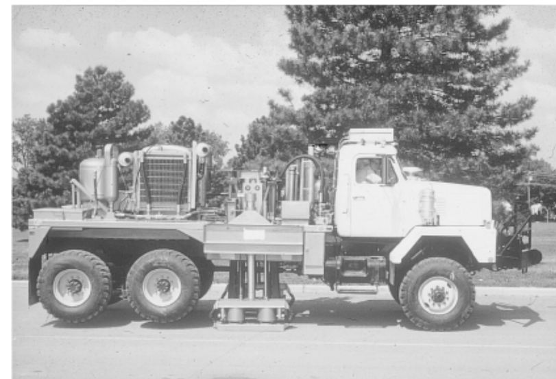
A Vibroseis truck, with massive hydraulic loudspeakers, transmits sound waves into the ground.
