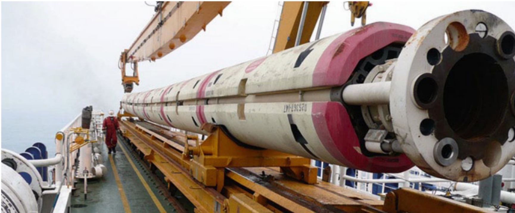
Fig. 4.4 A string of marine riser pipe. Note the small pipe openings embedded in the riser collar. These small pipes are used to control the well (“choke” and “kill” lines), and deliver hydraulic fluid to the BOP rams and LMRP annulars. In addition, the riser pipes carry power and electronic communication with the well. (Image source: Wikipedia)
