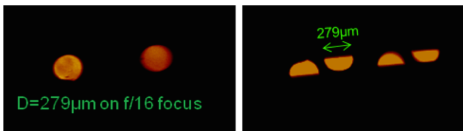
Figure 4 Example of a classical image slicer based on Bowen-Walraven prism (Giano-TNG spectrograph, first light prelist system)
