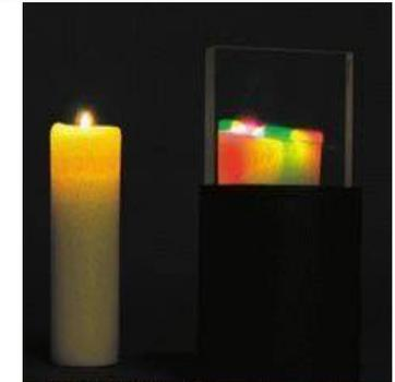
FIGURE 1. Multiplex volume-phase holographic grating is illuminated by candlelight. Two spectra are visible, one formed by each of the two gratings contained within the element. The shorter spectrum arises from the 1200-l/mm grating component and the longer from the 1620-l/mm component.
