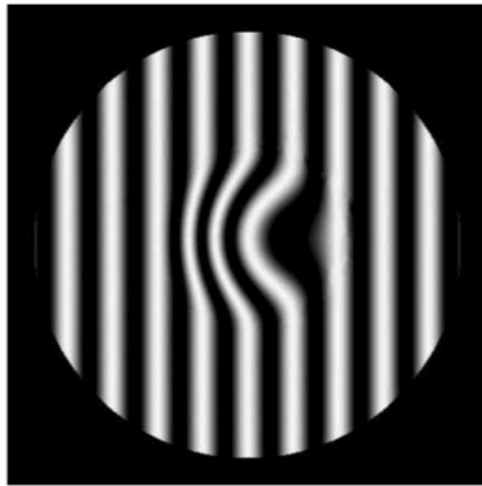
FIGURE 1.22. Kink formation in the straight Fizeau fringes of a slightly wedged plate, obtained by locally heating the plate. The kink is pointing toward the thin side of the wedge.
