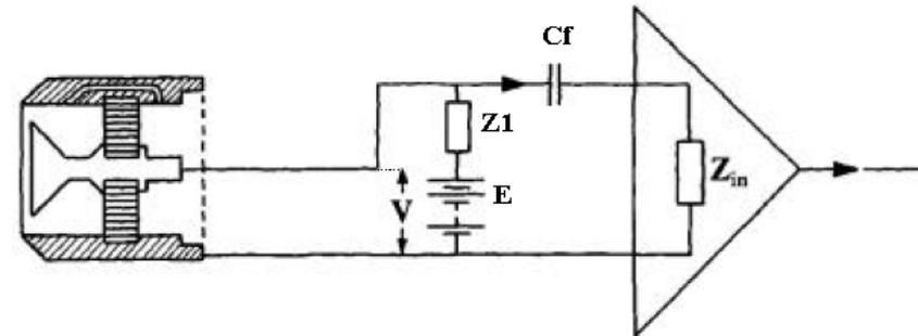
$$\left. \begin{aligned} Q &= CV \\ C &= \epsilon \frac{A}{d} \end{aligned} \right\} \Rightarrow V = \frac{Q}{C} = \frac{Q}{\epsilon A} d \Rightarrow \Delta V = \frac{Q}{\epsilon A} \Delta d$$
