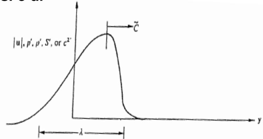
Fig. 1.1 Propagating disturbance.
