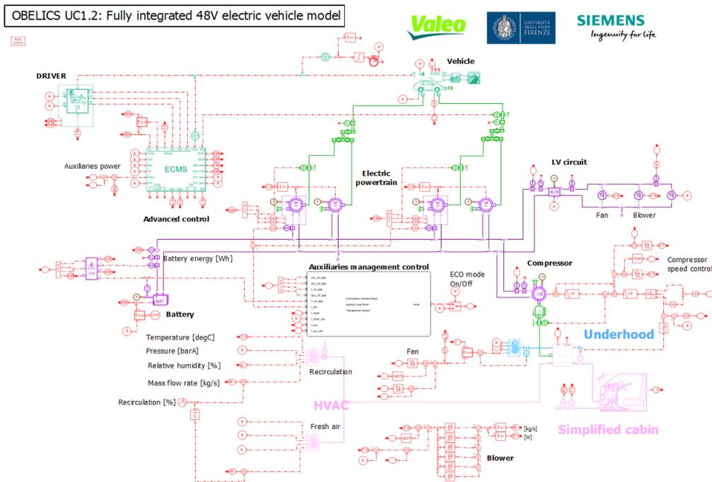
Fig. 4. Fully integrated 48 V electric vehicle model
