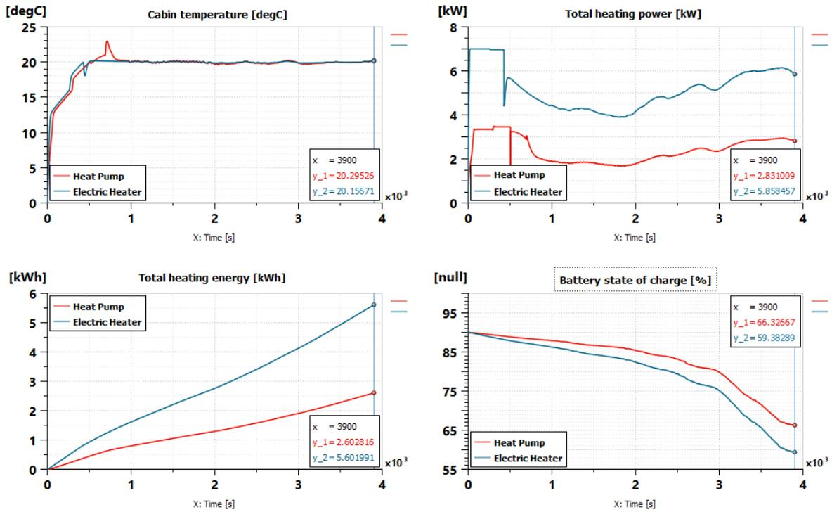
Fig. 5. Thermal system solutions comparison on ARTEMIS cycle: Cabin temperature (top-left); Heating power (top-right); Heating energy (bottom-left) and SOC (bottom-right)
