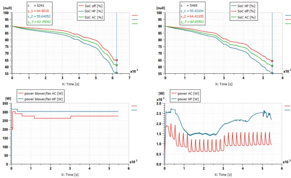
Fig. 6. Comparison on RDE Gratz (right) and Barcelona (left) at different ambient temperature: SOC (top) and thermal system power (bottom)
