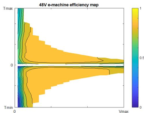
Fig. 2. 48 V e-machine efficiency map
