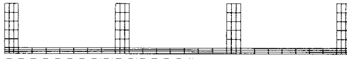
Figure 10.25. Mesh for an axisymmetric finite element model of the rotor in Examples 10.5.1 and 10.6.1.
