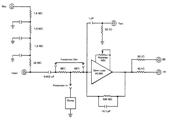
Fig. 4.1. Simplified Block Diagram of the 142PC Preamplifier.
