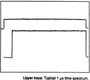
Lower trace: Same as above with STOP INHIBIT set to approximately 10% of full scale.
