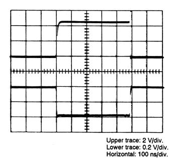
Figure 5 Typical SCA Output Pulses
