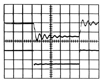
Uppe trace: Ungrounded Scope Probe Lower trace: At scope without proper termination Vertical at 0.5 V/div Horizontal at 100 ns/div.
