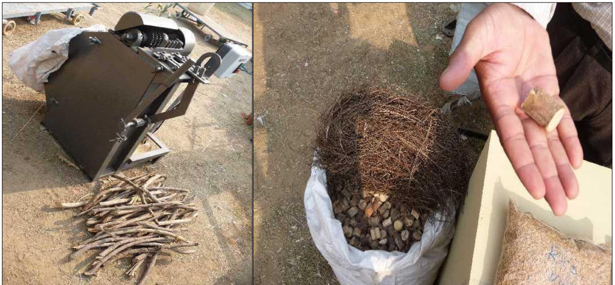
Figure 10. The small machine for cutting the lengths of woody weeds or jungle vine, and the cut product ready for fuelling the gasifier
