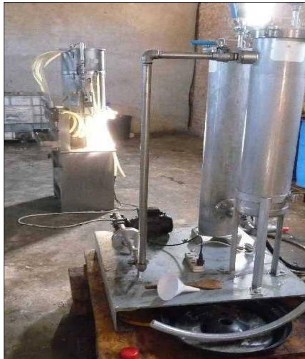
Figure 7. Crude jatropha oil filtering systems in use in Zambia to produce oil clean enough for fuelling modified diesel motors (in pumps and generators) and vehicles
