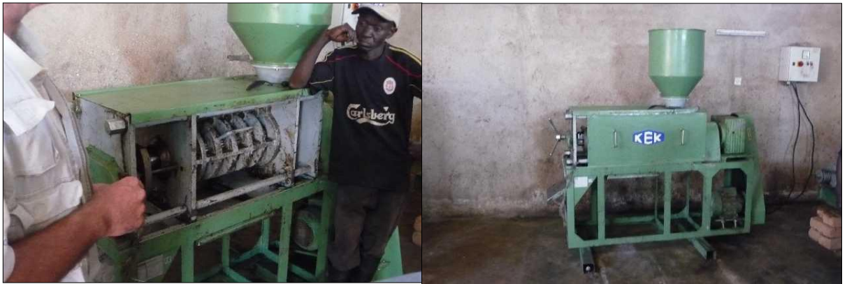
Figure 6. Small jatropha oil extraction machinery being used in Zambia
