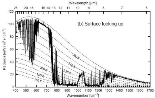
Figure 1. Coincident measurements of the infrared emission spectrum of the cloudfree atmosphere at (a) 20km looking downward over the Arctic ice sheet and (b) at the surface looking upwards. (Data courtesy of David Tobin, Space Science and Engineering Center, University of Wisconsin-Madison. Diagram courtesy of Grant Petty, from Petty 2006).
