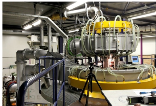
Non-Rotating Annular Test Facility dedicated to turbomachinery aeroelastic investigations, DLR Göttingen (formerly EPFL Lausanne)
