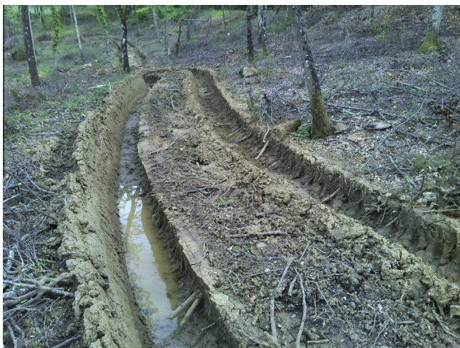
Fig. 1. Ruts created by a wheeled tractor during logging operations in the silt loam soil of a coppice oak forest in the Chianti region, Tuscany, Italy. Visible damage includes broken roots, soil displacement and compaction. Soil compaction is so extreme that water does not percolate into the soil and induces anoxic conditions in the top layer. During the rainy season, ruts become preferential flow paths and result in erosion.
