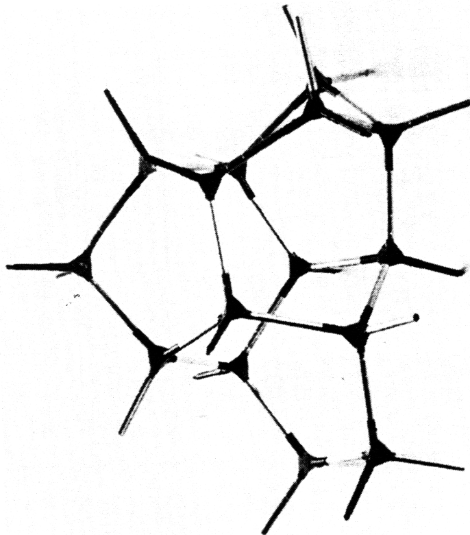
Figure 5-31. Polk model for the structure of a -Si. Five-membered rings may be seen at the top (atoms 10, 11, 13, 14, 15) and lower right (atoms 3, 4, 5, 12, 7). A six-membered ring in "chair" configuration is on edge at the right (atoms 4, 5, 6, 11, 12, 13). "Boat"-configured six-membered rings are at the left (atoms 1, 2, 10, 15, 8, 9 and atoms 7, 3, 2, 8, 15, 10).
